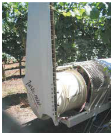
Spray tower reduces pesticide drift NIELS HOLBEK PHOTO
